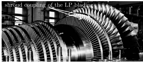
Fig. 1 Low pressure steam turbine blading with a shroud coupling (courtesy of Siemens AG-Energy Sector)
